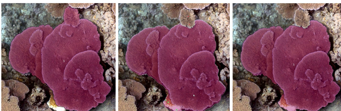
FIGURE 17 Edit a colony using the positive/negative clicks tool. The original form (left). Drawing negative points in red excludes an area. Drawing positive points in green includes an area. Using automatic refinements further improves segmentation (right) [Color figure can be viewed at wileyonlinelibrary.com ]
