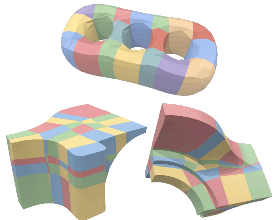
Fig. 13. The Hole3 model decomposed in eighteen parts (top) and the Fandisk model decomposed in fifty parts (bottom).
