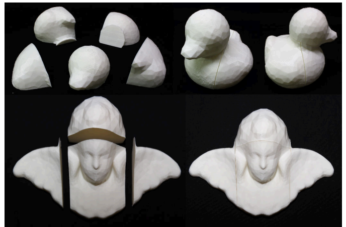
Fig. 10. The models of Duck and Angel . On the top left the five printed parts of the Duck , and on the top right two views of the assembled model. On the bottom left the four parts of the Angel , and on the bottom right the assembled model.
