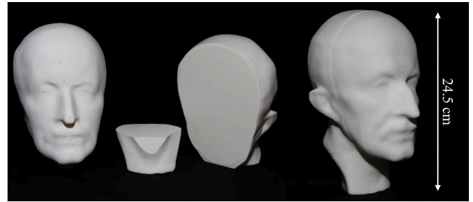
Fig. 12. The Max Planck model fabricated. The three separated parts on the left, and the assembled model on the right.
