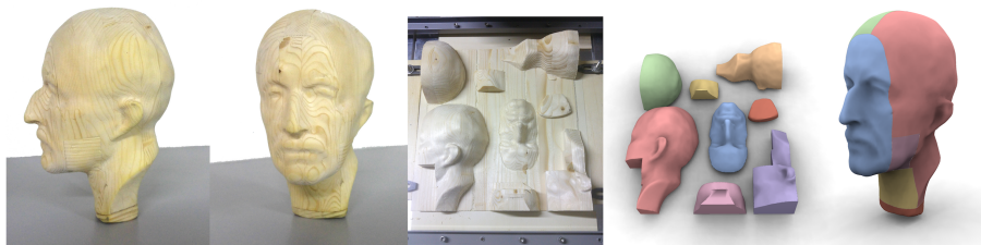
Figure 1.4: We enable fabrication of general 3D geometries (right) using single pass 3-axis CNC machining by algorithmically decomposing 3D geometries (left) into height-field blocks (center).
