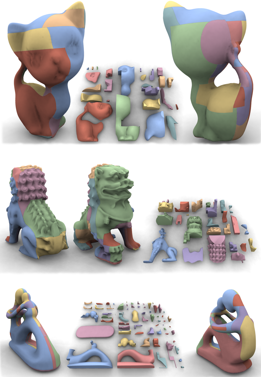
Figure 4.9: Our method produces valid, compact decompositions for complex models containing: non-trivial topology (e.g., Fertility), thin features (e.g., the ears of the Kitten) and large portions not aligned with the global frame (e.g., the Chinese Lion’s body) for which manual decomposition is highly challenging to compute, resulting in 27 blocks for the Chinese Lion, 25 for Kitten and 63 for Fertility.
