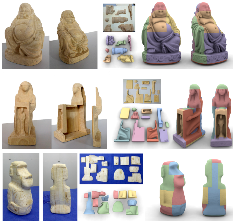
Figure 4.10: A gallery of decompositions computed with our algorithm and fabricated in wood using a 3-axis milling machine.
